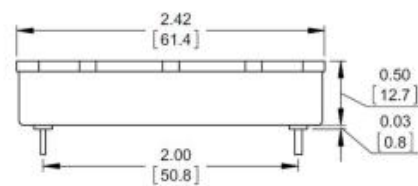
Shape – WB (Base Plate with DOSA pinout)
